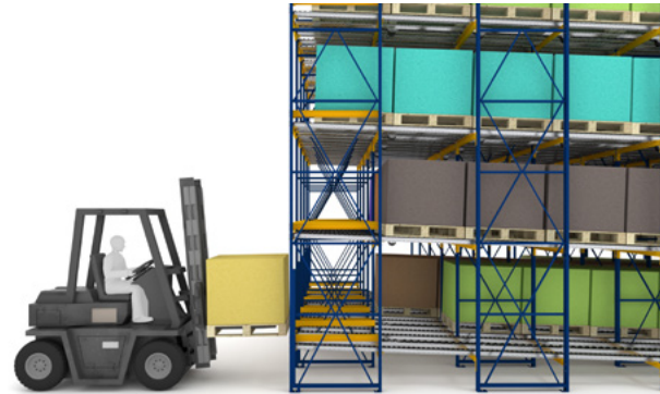
Square the forklift with lane & raise the pallet 3" above the rails
