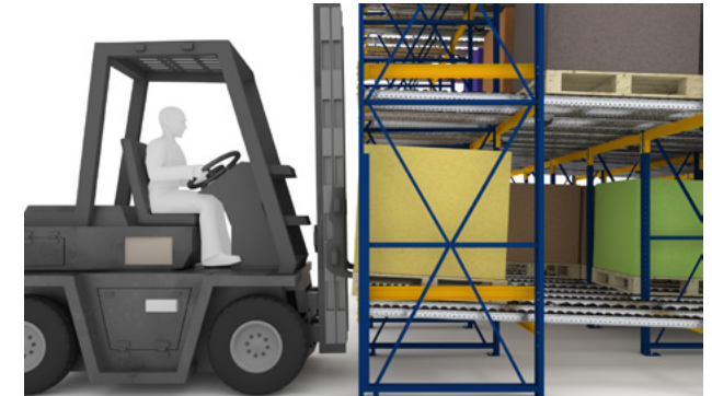
Place the pallet centered in the lane & tilt onto the rails
