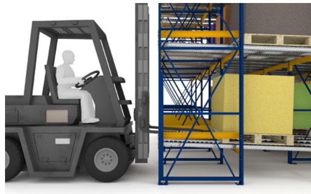
After placing the pallet, slowly back out of the lane
